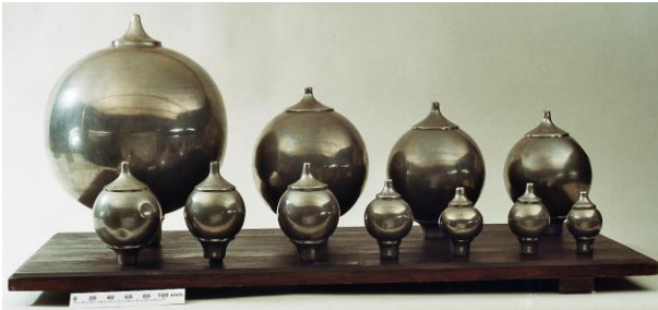
Figure 2: Set of Helmholtz resonators, Leppin & Masche, Berlin 1913 (HAPS Dresden).
