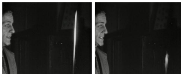
Figure 3: Dipping of the sensitive flame, probably in response to a sibilant. The two images shown are 7 frames apart on the film (about 350 ms).
