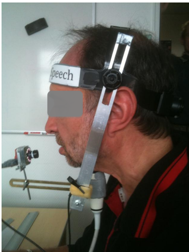
Figure 1: Acquisition helmet worn by post-laryngectomy volunteer; ultrasound transducer beneath the chin; 60 fps lip camera with IR illumination; lapel microphone (clipped to aluminum strut). Tracheostoma is visible to right of transducer.
