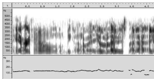
Fig. 5. Wide-band spectrogram of RUDLAD's third utterance after seizure, showing octave errors by pitch tracker.
