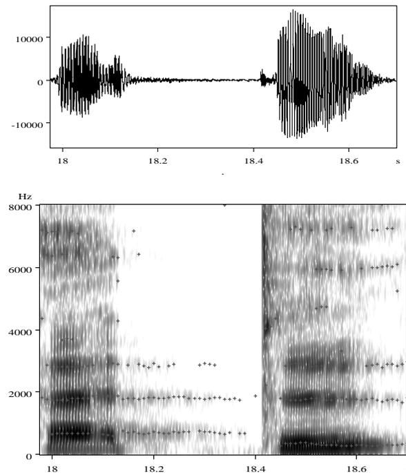
Figures 3A and 3B : Signal and sonogram produced by patient #5 during the [ati] sequence. The crosses on the sonogram represent the formant obtained after an LPC analysis.
